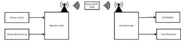
Figure 2. System block diagram of the wearable monitoring prototype.
